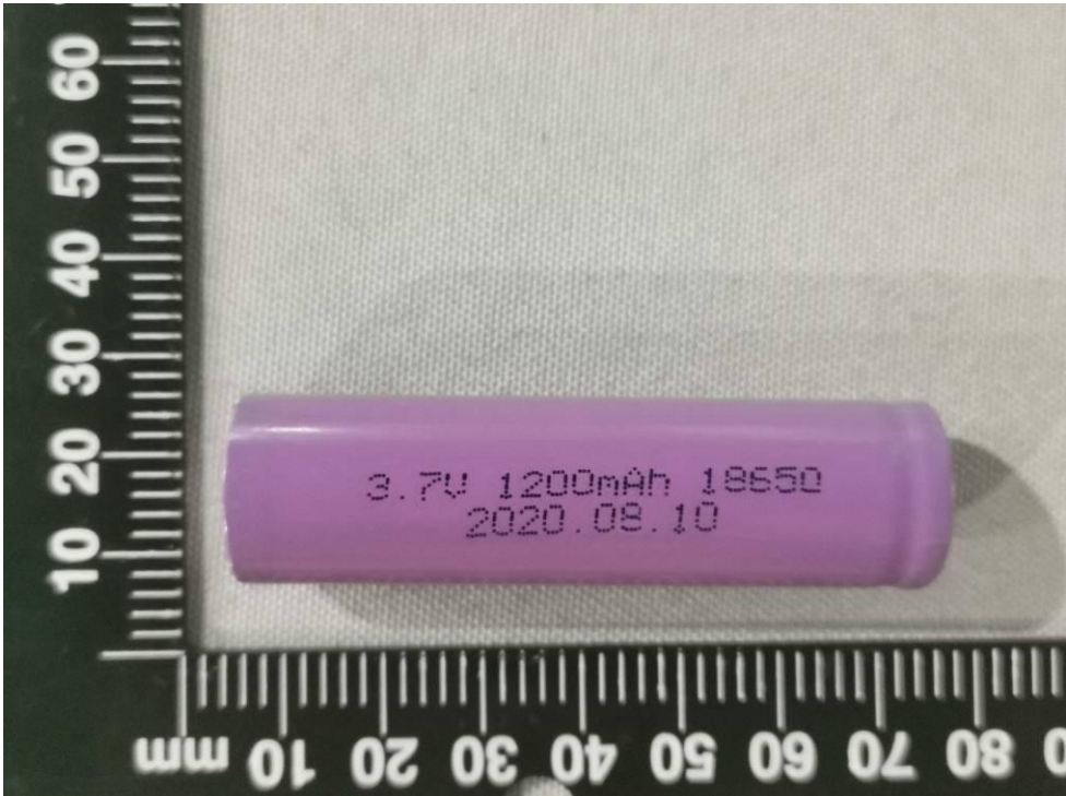
Cell (18650 3.7V 1200mAh 4.44Wh)
